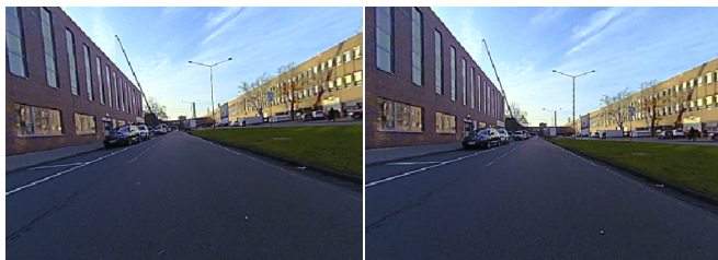
Fig. 6. Planar unwarping, 100-degree horizontal field of view; left: surface not aligned to vehicle; right: surface aligned to vehicle
