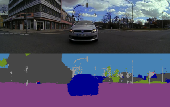
Fig. 2. Cylindrically unwarped rear image and segmentation results
