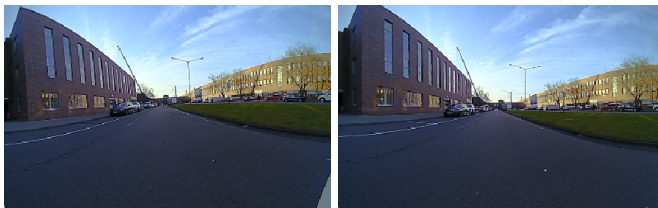
Fig. 7. Cylindrical unwarping, 160-degree horizontal field of view; left: surface not aligned to vehicle; right: surface aligned to vehicle
